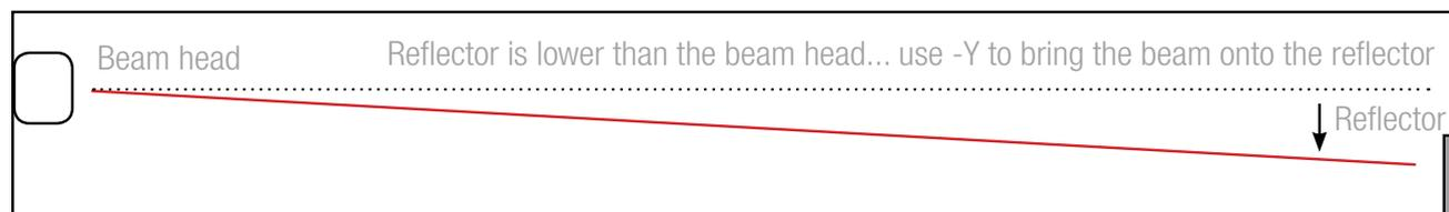
The beam can be moved on both X and Y axis to a maximum 5 degrees using the **left (x-), right (x+), up (y+) and down (y-)** keys. Looking at the reflector this will move the beam across the reflector like so...
