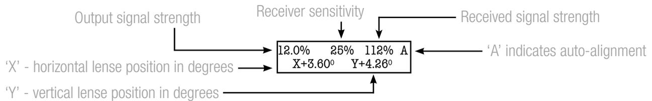
Auto alignment in 'fast' mode will take, on average, 3 minutes and in normal mode up to 30 minutes the better the beam is aligned before auto alignment (high AQ readings) the shorter the align time. Once finished **Align Complete** will appear on the screen, simply press **left back** to OK and exit.
