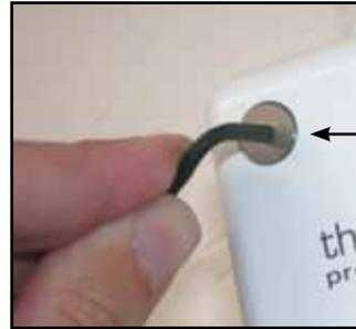
Screw the head screws down with the 3mm allen key provided. **Your wiring should be flush and not flattened by tightening down screws.**
