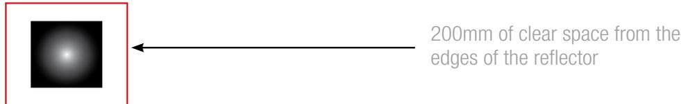
Once the reflector is in place and visible there should be a big jump in the received signal (AQ). This means that the head is seeing and receiving a signal back from the reflector. In most cases this will result in a received signal of over 100%.
